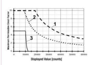
Additional error caused by signal's crest factor: 1 < CF < 3: 1% R+ 30D 3 < CF < 10: 3% R
