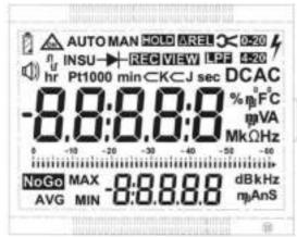
LCD display field 67 mm X 54 mm with digital display, analog scale and with display of measurement unit, and Various special functions.
