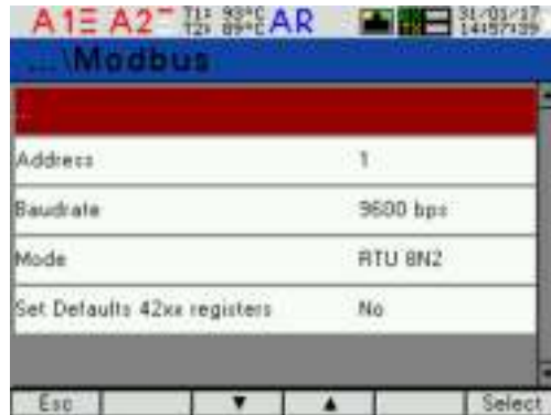
Fig.21. Screens of Modbus group
