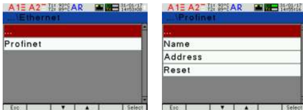
Fig.20. Screens of Ethernet / Profinet group
