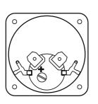
This is available as a rear mounted factory fitted option. The unit contains a Ø 6mm 'festoon' style lamp available in 6V, 12V or 24V. Please contact the sales office for more
