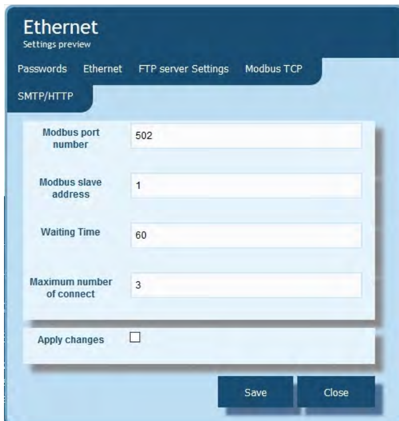
Fig. 21 View of Modbus TCP configuration parameters on "Ethernet" tile
