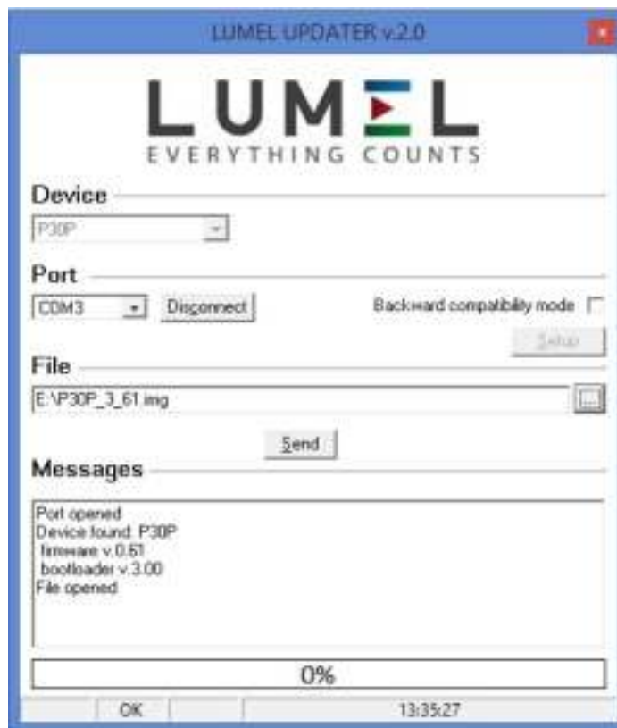
Fig.18 View of the program for updating transducer software.
