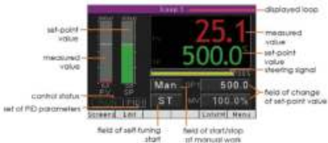
Fig. 6. Screen with fixed set-point control
